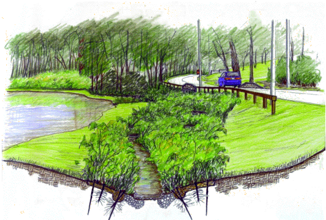
Figure 4.34 - Example Route 100 in Delaware, illustrating ideas for better roadside details for drainage – using soil-bioengineering instead of rip-rap
